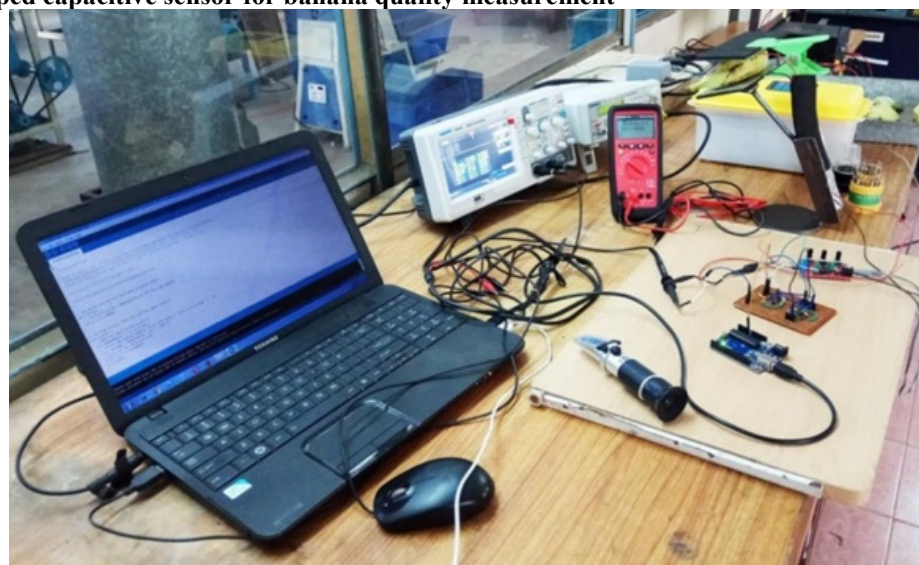
Fig 3. Developed capacitive sensor for banana quality measurement
